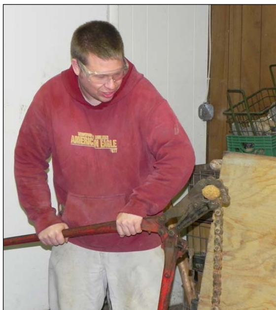
■ Patrick Pierce demonstrated how to use the pipe snap cutter at the October Club Work Day.
