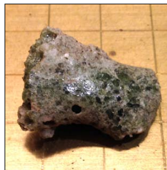
To further explore extreme blast dynamics, Randy Patrick will conduct tests on this piece of Trinitite, glass material formed by the 1945 Trinity nuclear test in New Mexico. photos courtesy of Randy Patrick
